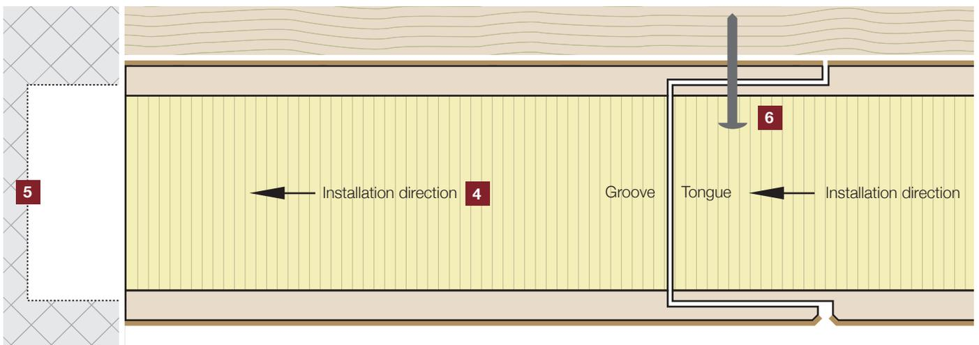
**4 Observe the installation direction: work “tongue in groove” (GROOVE ← TONGUE)**
