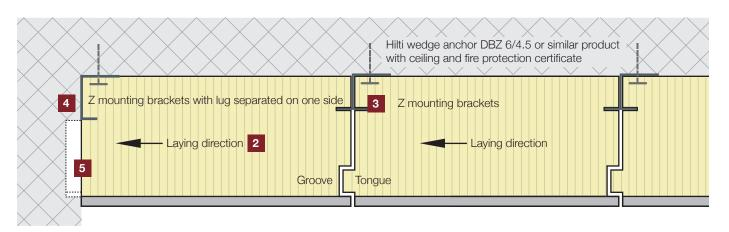
Two Z mounting brackets are used per panel.
