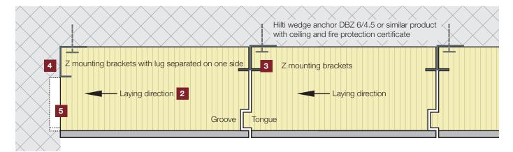
Two Z mounting brackets are used per panel.
