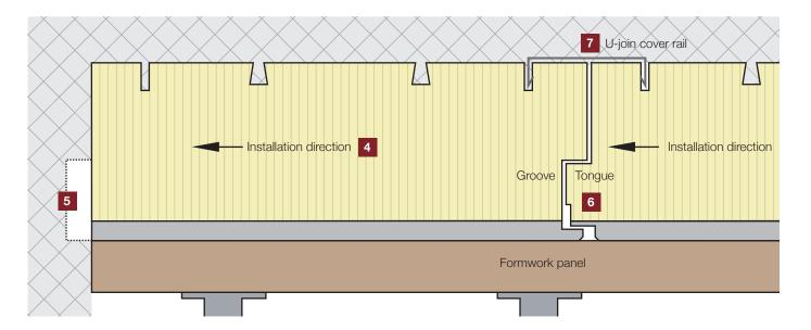
Always work "tongue in groove" to prevent any dirt from depositing beneath the tongue that may prevent a closed join. It is especially important to always start with the tongue pointing towards the outer wall. A different kind of installation may lead to protrusions of the joins on the surface that are visible later on and cannot be corrected retrospectively.
