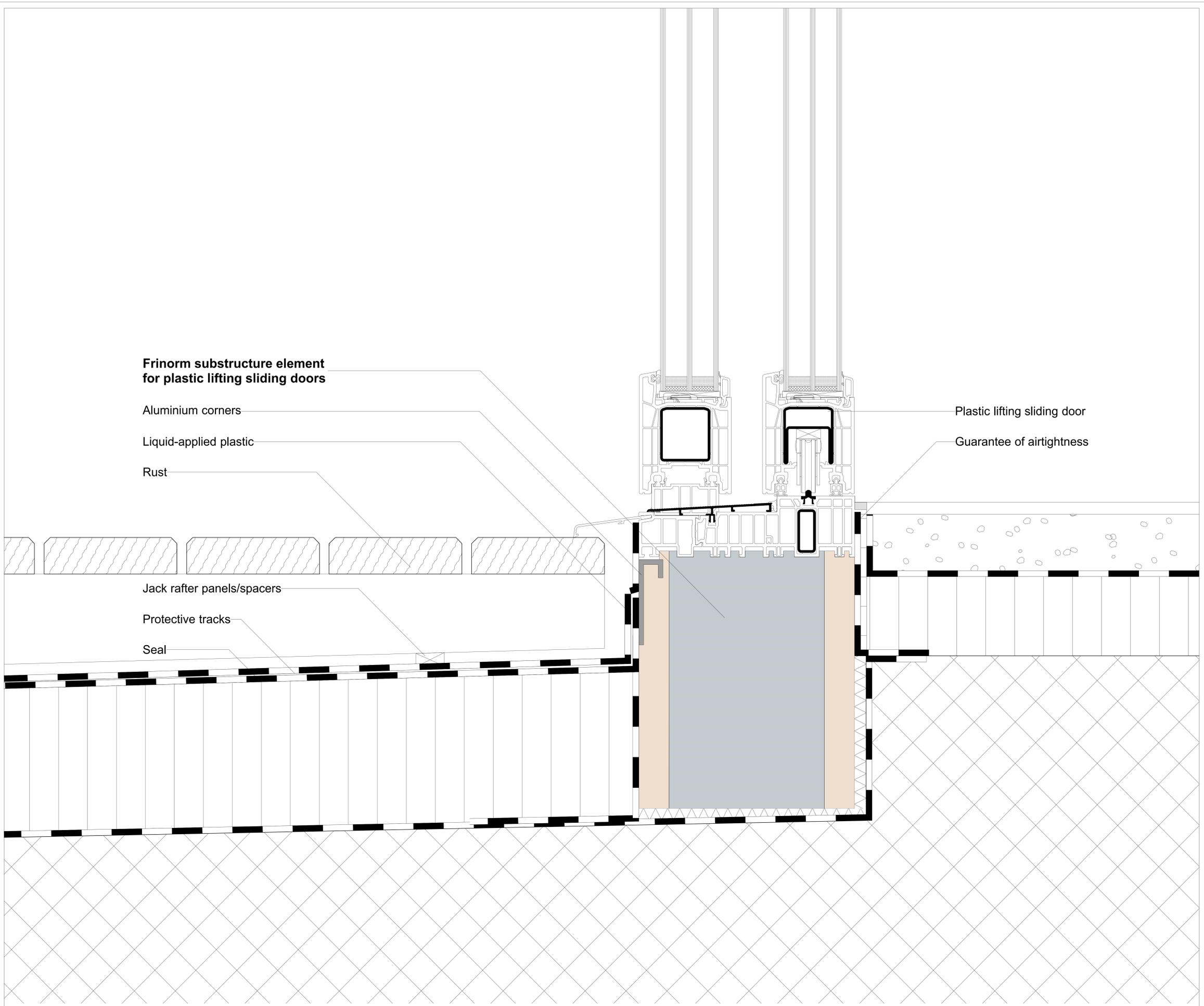
**Threshold detail plastic lifting sliding door**
